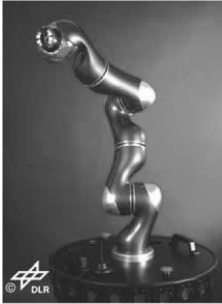
Fig. 3.38. Advanced dexterous manipulator arm for space applications developed at DLR.
