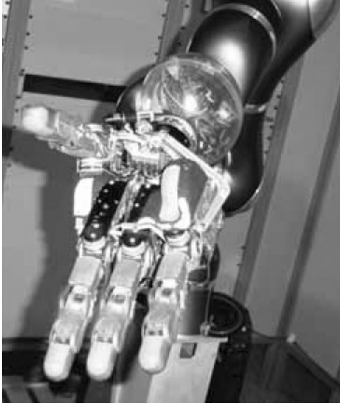
Fig. 3.39. Dexterous four-fingered hand developed for space applications at DLR.
