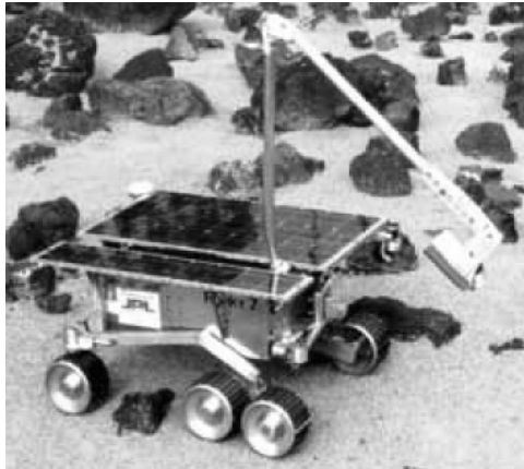
Fig. 3.24. Rocky-7 Rover, developed by JPL for long-range traverse in a Sojourner-sized vehicle.
