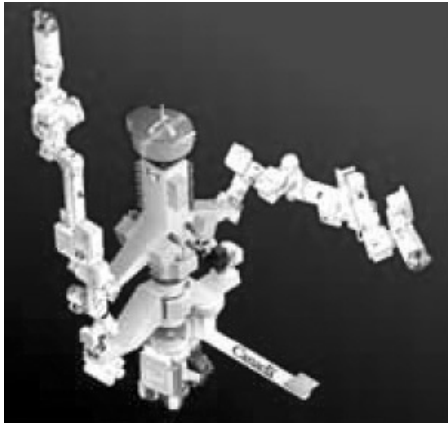
Fig. 3.28. Special-purpose dexterous end-effector, developed by McDonnell-Detweiler Robotics for the Canadian Space Agency.
