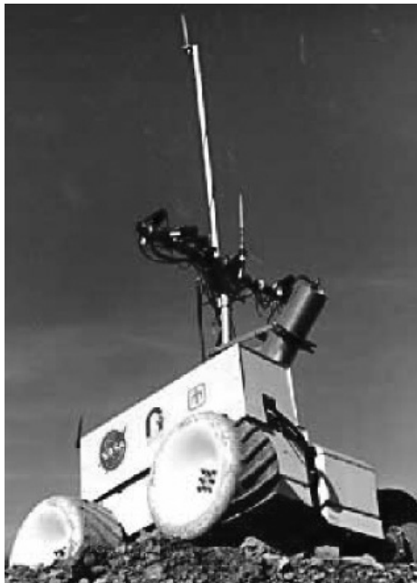
Fig. 3.20. RATLER Rover developed jointly by Carnegie-Mellon University and Sandia Laboratory for use on the Moon.
