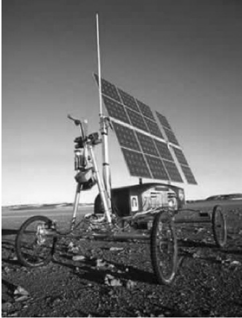
Fig. 3.21. Hyperion robot developed by Carnegie-Mellon University used in arctic and other planetary analog sites.
