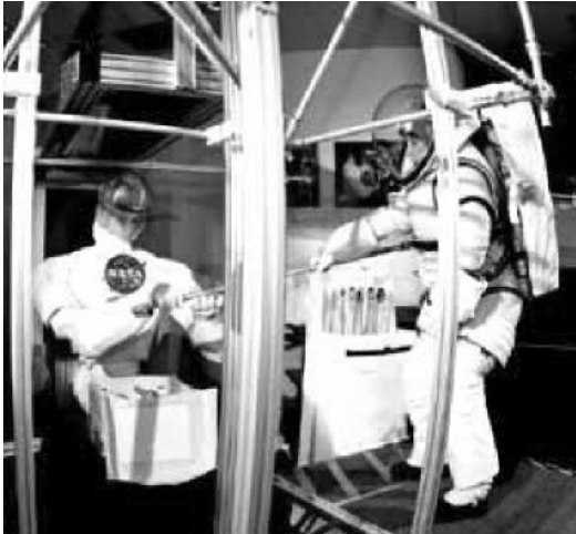
Fig. 3.10. Robonaut engaged in cooperative truss assembly task with human astronaut in lab.
