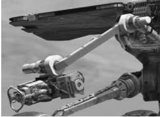
Fig. 3.29. Mars Exploration Rover robot arm, developed by Alliance Spacesystems, Inc., for JPL.
