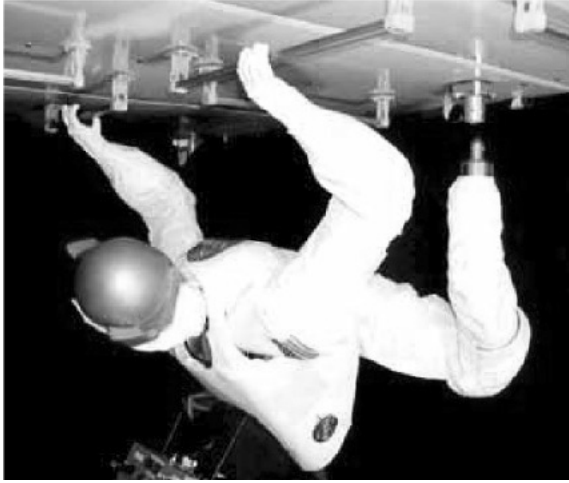
Fig. 3.9. Robonaut using handrails designed for human astronauts in simulated zero- g (using air-bearing floor).
