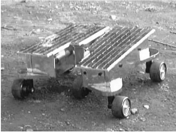
Fig. 3.48. Development model of a lunar rover for the Japanese mission SELENE-II.
