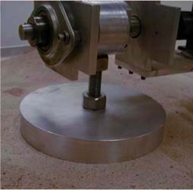
Bevameter (force vs. displacement)
