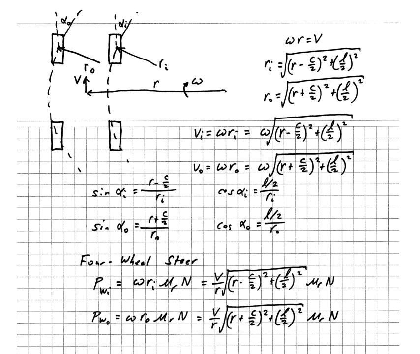
$$\frac{P_{skid}}{P_{steer}} = \frac{\frac{V}{r} \left[ \frac{d}{2} u_r + (r + \frac{c}{2}) u_s \right] N}{\frac{V}{r} \sqrt{(r + \frac{c}{2})^2 + (\frac{d}{2})^2} u_r N} = \frac{\frac{d}{2} + (r + \frac{c}{2}) \frac{u_s}{u_r}}{\sqrt{(r + \frac{c}{2})^2 + (\frac{d}{2})^2}}$$
