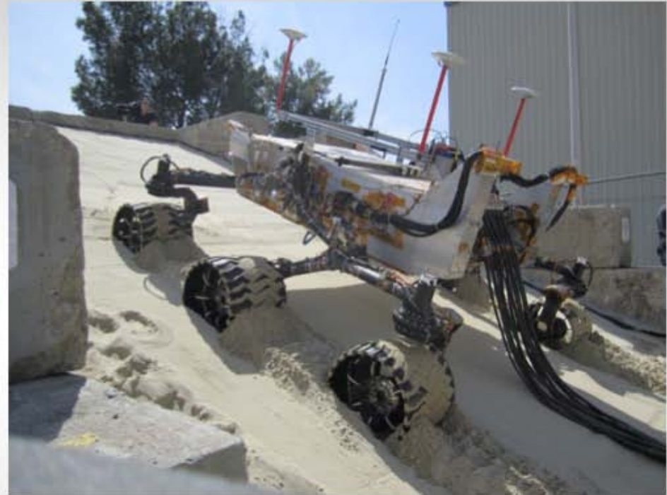
NASA's Mars Science Laboratory (MSL) Design/Test Model (DTM) in the sandy Mars Yard at JPL
