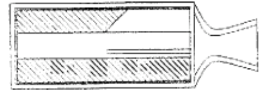
Slots and tube (case bonded), neutral burn
