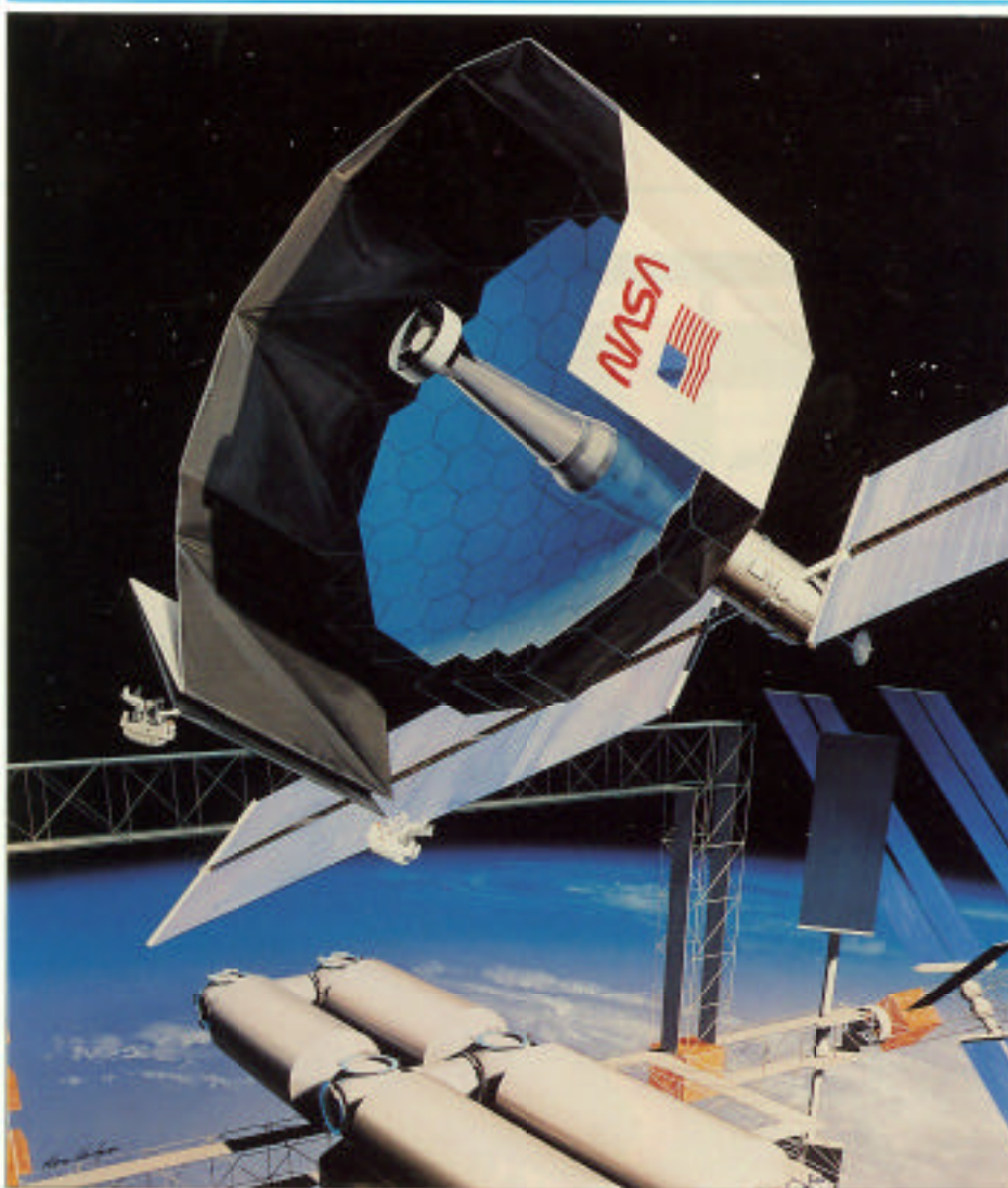
LDR, with 20-meter mirror and sunshade, during assembly at the Space Station facility.
