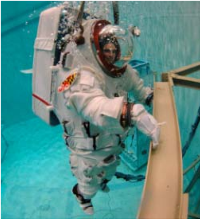
Figure 10: The MX-2 neutral buoyancy space suit analogue. Note the large HUT, which will be modified into a Soft/Hard Upper Torso.
