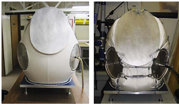
Fig. 5. Full scale MUT model in expanded state (left) and reconfigured to nominal configuration (right).
