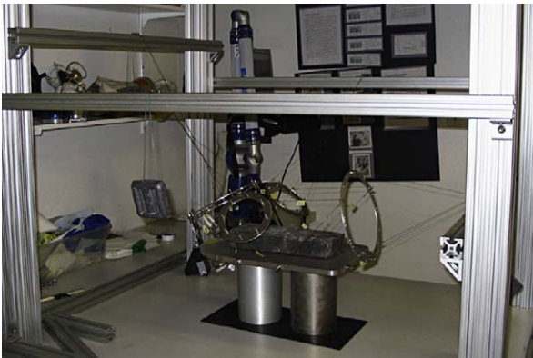
Fig. 4. Experimental model for the isolation of pressurized fabric effects.
