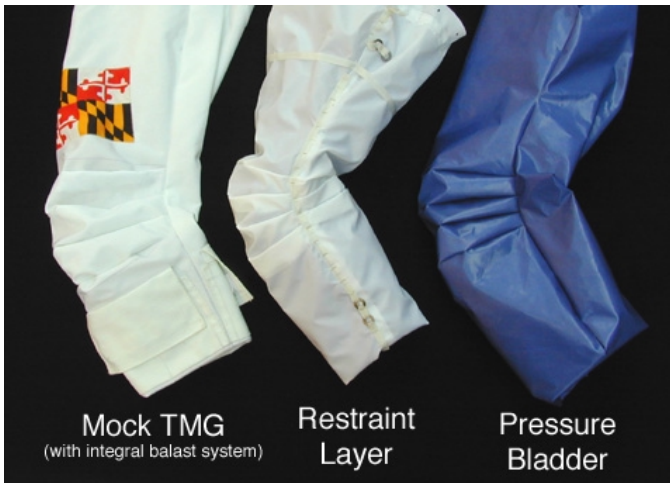
Figure 3. The 3 layers that make up the new soft goods used on the MX-2.
