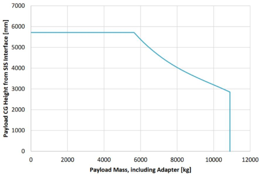
Figure 3-2: Allowable center-of-gravity height above the 1575-mm plane
