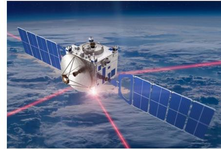
Figure 1 - Small Communications Satellite with Deployed Solar Arrays
