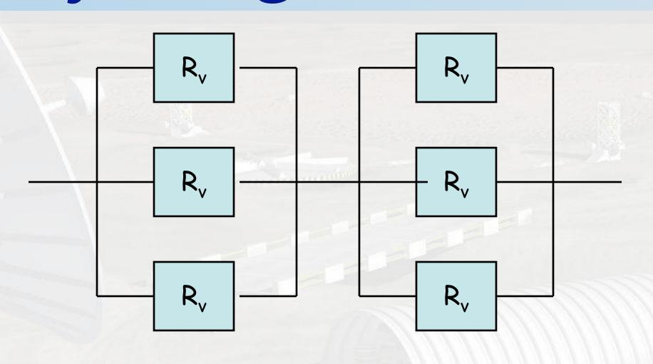
$$R_{\text{system}} = \left[1 - (1 - R_{\text{v}})^{3}\right]^{2}$$
