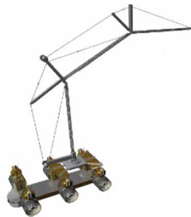
Figure 3. The Lunar Surface Manipulator System mounted to the top of a crew mobility chassis to maximize the range of unloading from Altair.
