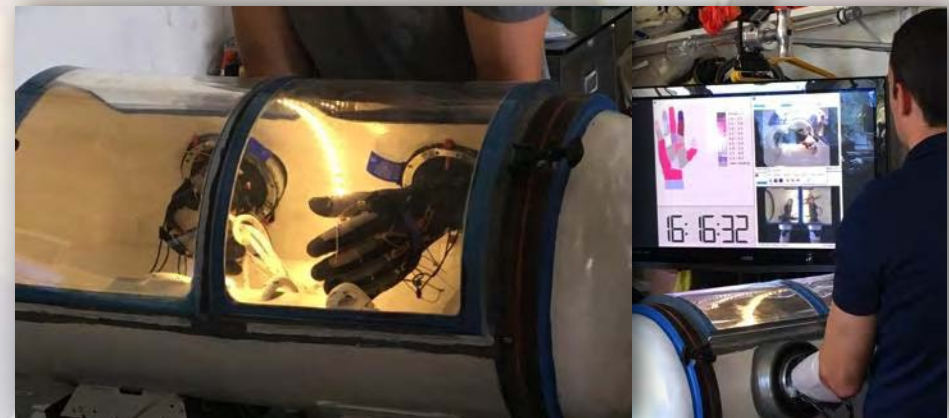
Glovebox Testing of Mechanical Counter Pressure Prototypes
