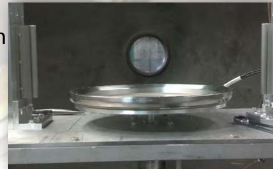
Hip bearing test set-up in WSTF chamber
