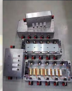
Power load boxes
