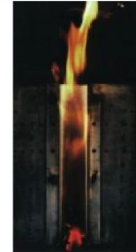
Sample failing NASA Test 1
