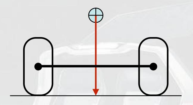
Rover is stable so long as gravitational force vector passes inside the stability region formed by the contact points of the suspension with the ground
