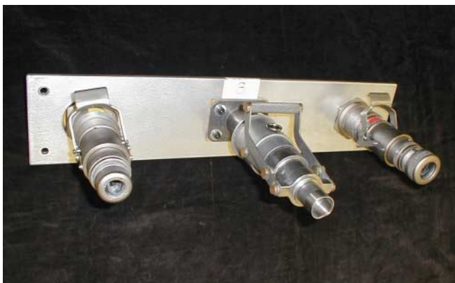
ISS Hydraulic and Electrical Connectors Figure 7
