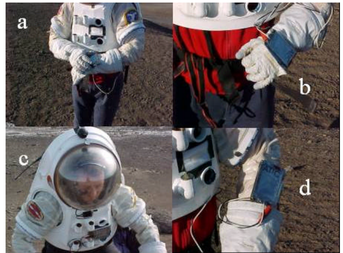
Figure 8: Alternative mounting locations for mouse pad a) top of hand, b) wrist, c) front of HUT, d) forearm.
