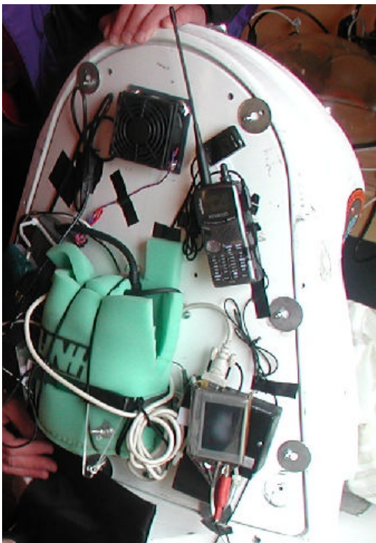
Figure 3: Rear view of the simulator showing CPU, optical display system, video converter box, brushless DC motor, batteries, mouse pad, GPS, and two way radio.
