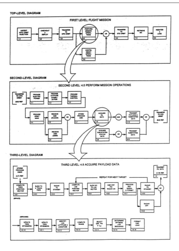
Figure B-6 — Development of Functional Flow Block Diagrams.
