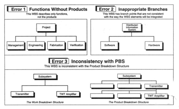
Figure 11 — Examples of WBS Development Errors.
