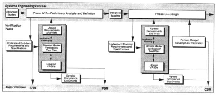
Figure 32a — Verification Process Flow (Phases A/B and C).
