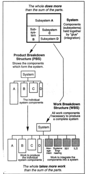
Figure 10 -- The Relationship Between a System, a Product Breakdown Structure, and a Work Breakdown Structure.
