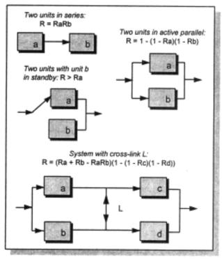
Figure 29 — Basic Reliability Block Diagrams.
