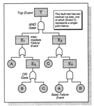
Figure 30 - A Simple Fault Tree.
