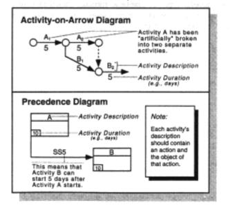
Figure 12 — Activity-on-Arrow and Precedence Diagrams for Network Schedules.
