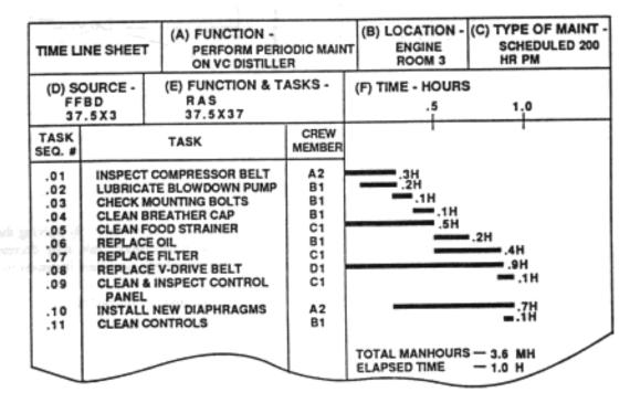
Figure B-10 — Sample Maintenance Time Line Sheet.
