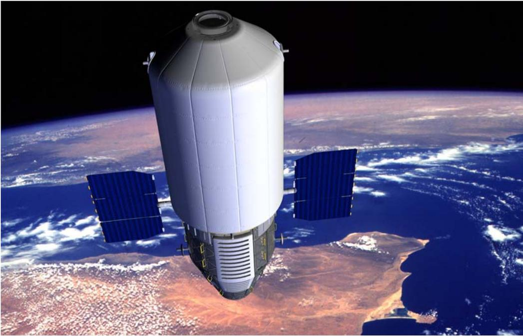
*Figure 5-1: Hybrid Propellant Module.*
