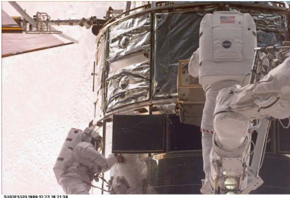
Fig. 2. Two-human crew replacing the fine guidance sensor on the Hubble Space Telescope (image from nasa.gov photo archives).
