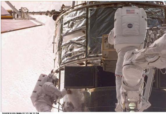
**Fig. 2.** Two-human crew replacing the fine guidance sensor on the Hubble Space Telescope (image from nasa.gov photo archives).
