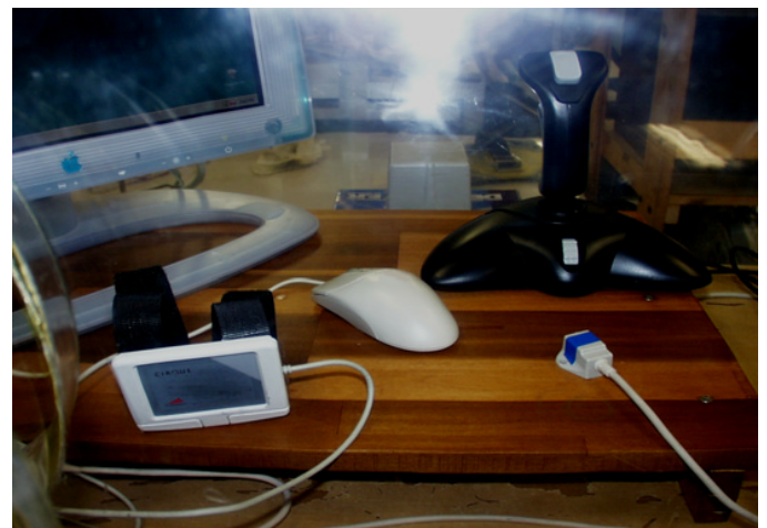
Figure 1: Hand Controllers Selected from L to R: Touchpad, Mouse, Joystick, Magnetic Motion Sensor.
